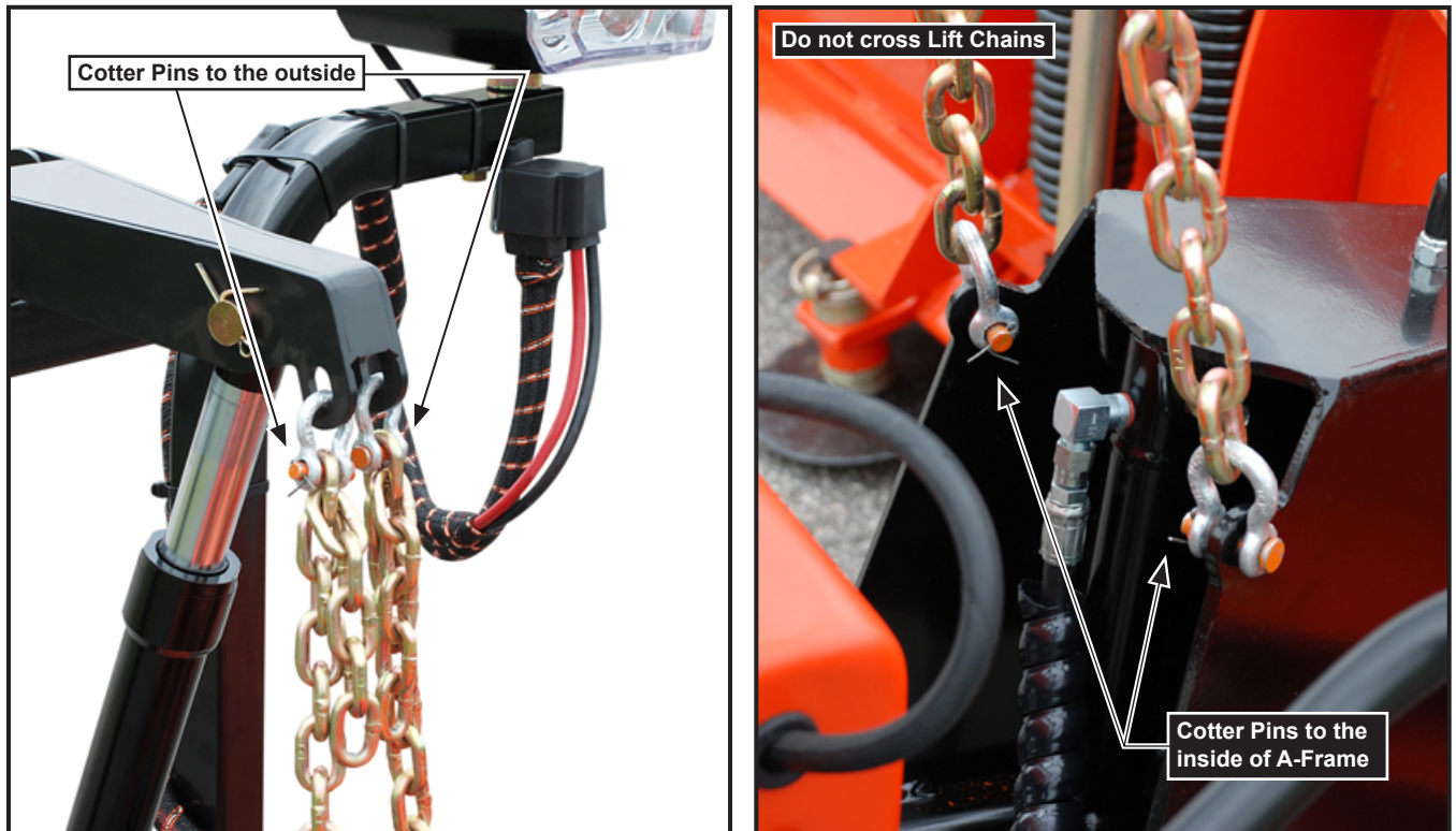
Figure 15. Lift Chains Installed
