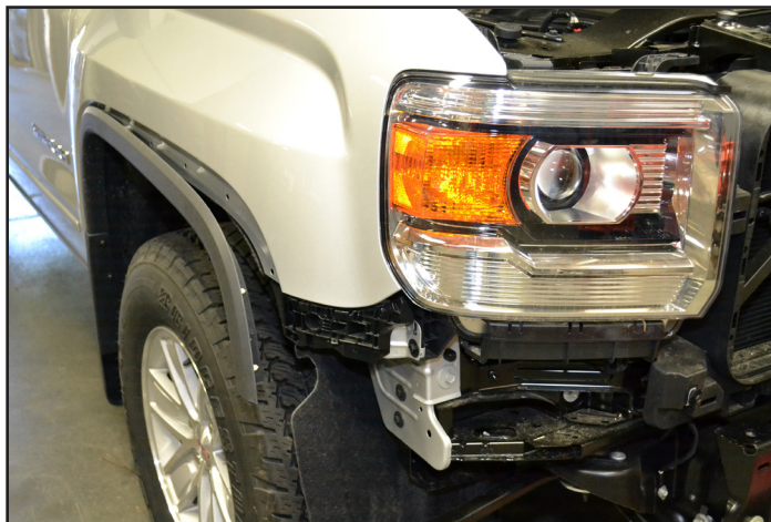
Figure 2. Grille and Bumper Bolt Locations
