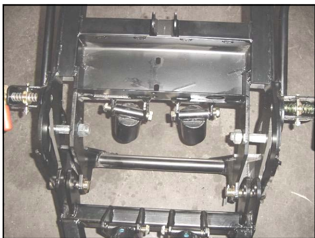
Fig. 5.2 (view of both upper spring cans installed)
